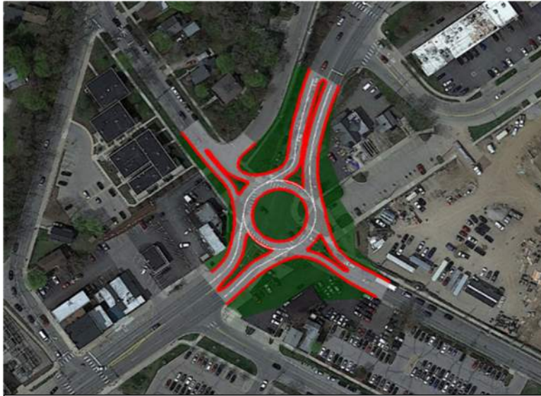
Convert intersection of Broadway St, Maiden Lane and Moore St to 2-lane roundabout. Moore St could change to 2-way traffic. Depicted is one with about 150' diameter.
