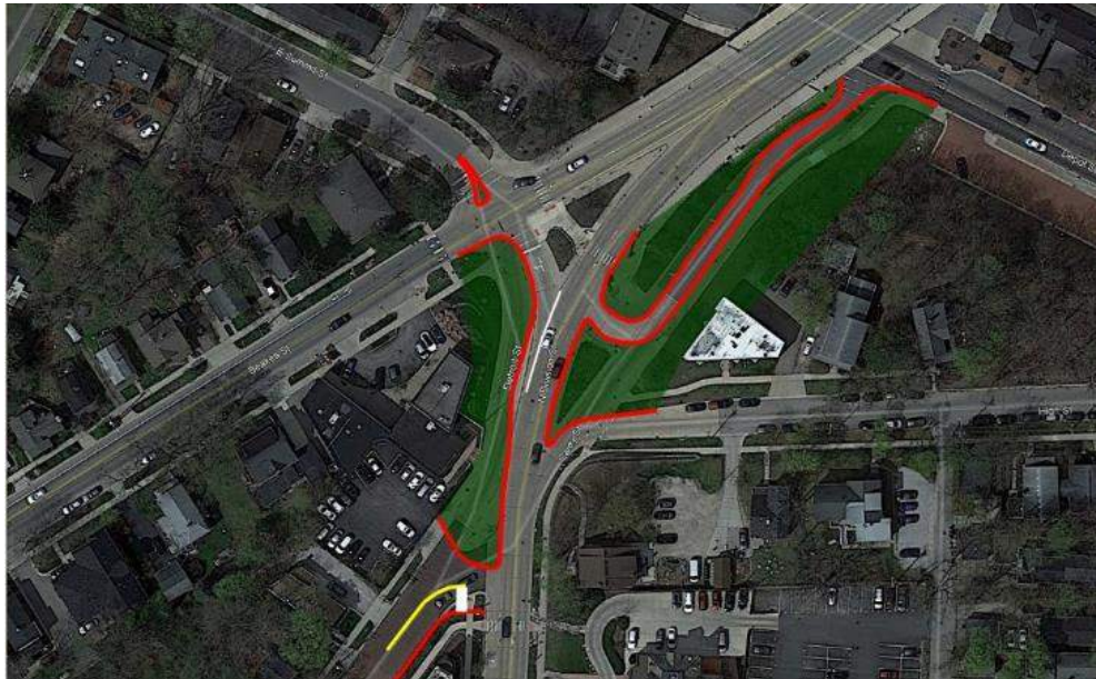
Option C – Close northbound entrance to Carey St from Division St and southbound access to Detroit St from Broadway St/Summit St. Maintains access from Division to Summit. Left turns and thru movements would be channelized. Would maintain access to the Broadway Street bridge from Depot Street and to High Street from Division.
