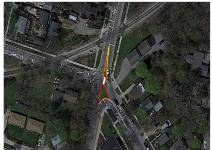
Mid-Term Option A – Add new islands to intersection. Stop sign would be added for Moore Street to Longshore Drive movement. Traffic flashers would be removed.
