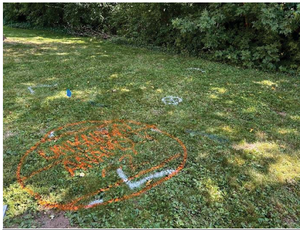
Picture 3: This image depicts our surface markings behind the building. The circled area is where the anomaly was located at a depth of 1'-2' that was found in Picture 2. There was also a waterline running through the scan area near the soil boring location.
