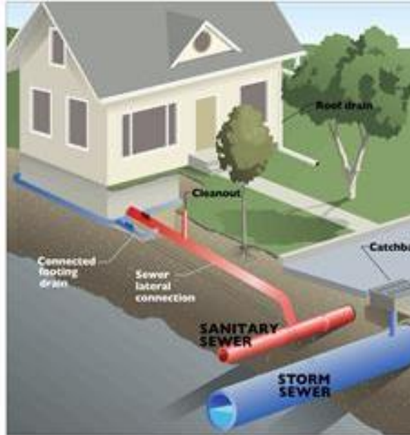
Reduced risk of basement back-ups
