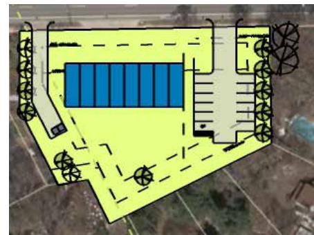
Figure 1.3 (2) - Site plan with rowhouses. Eight units max with parking lot on east.
