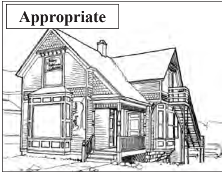
It is appropriate to preserve and maintain wood siding, trim and architectural details.
