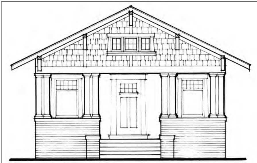
Preferred Approach when historical documentation is available: Craftsman style house with a replacement porch designed similar to that seen historically.
