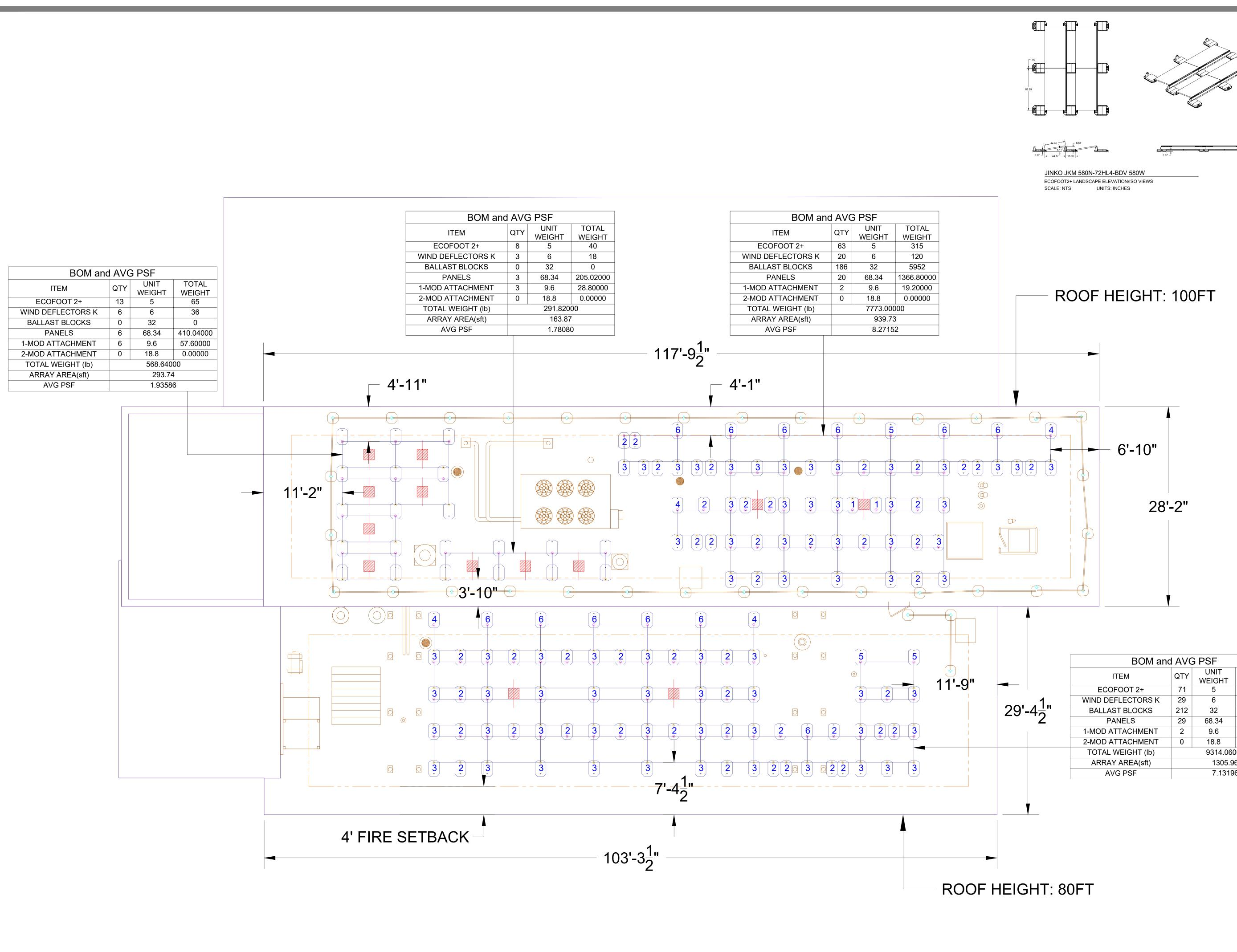
DRAWING INDICATES PLACEMENT OF EQUIPMENT AND BALLAST. PLEASE REFER TO INSTALLER IS RESPONSIBLE FOR VERIFICATION OF SITE AND PROJECT SPECIFICS. DESIGN IS FINALIZED WHEN ACCOMPANIED BY STAMPED ENGINEERING REPORT.
