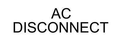
LABEL 10 EACH AC DISCONNECTING MEANS MUST BE LABELED WITH THIS PLACARD
