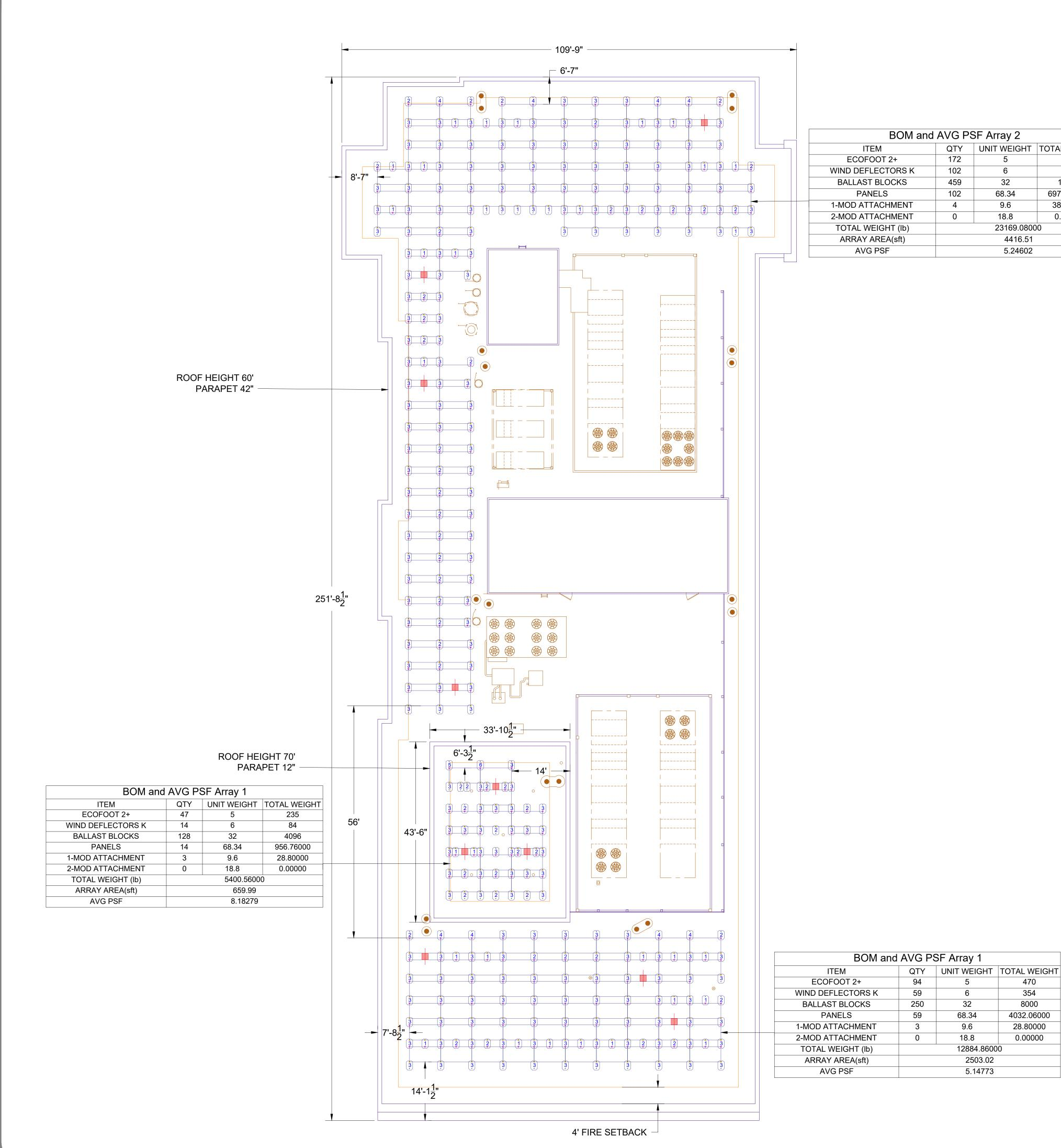
DRAWING INDICATES PLACEMENT OF EQUIPMENT AND BALLAST. PLEASE REFER TO INSTALLATION MANUAL FOR FULL PRODUCT DETAILS. INSTALLER IS RESPONSIBLE FOR VERIFICATION OF SITE AND PROJECT SPECIFICS. DESIGN IS FINALIZED WHEN ACCOMPANIED BY STAMPED ENGINEERING REPORT.
