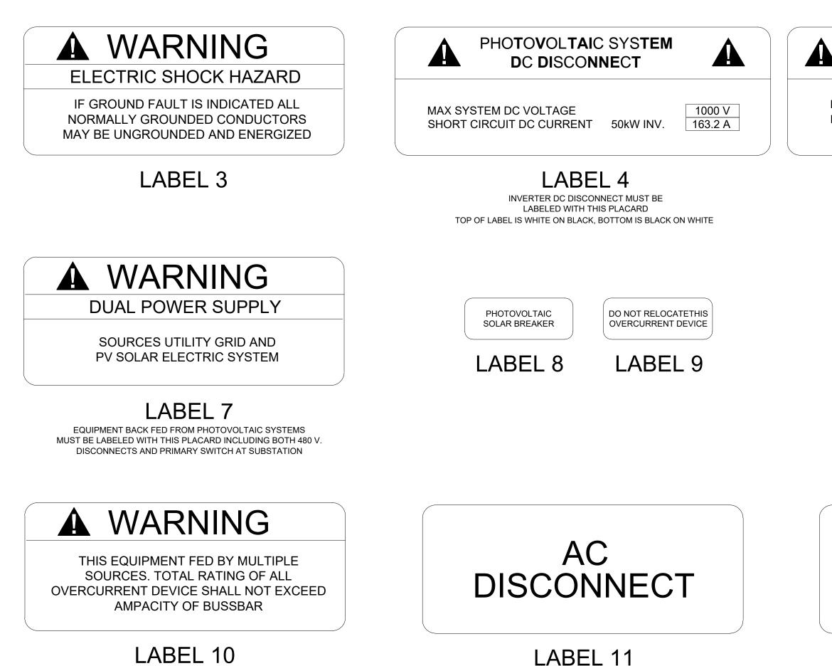
EACH AC DISCONNECTING MEANS MUST BE LABELED WITH THIS PLACARD
