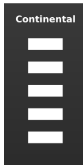
Figure 4.1.5- Crosswalk Pattern Markings
