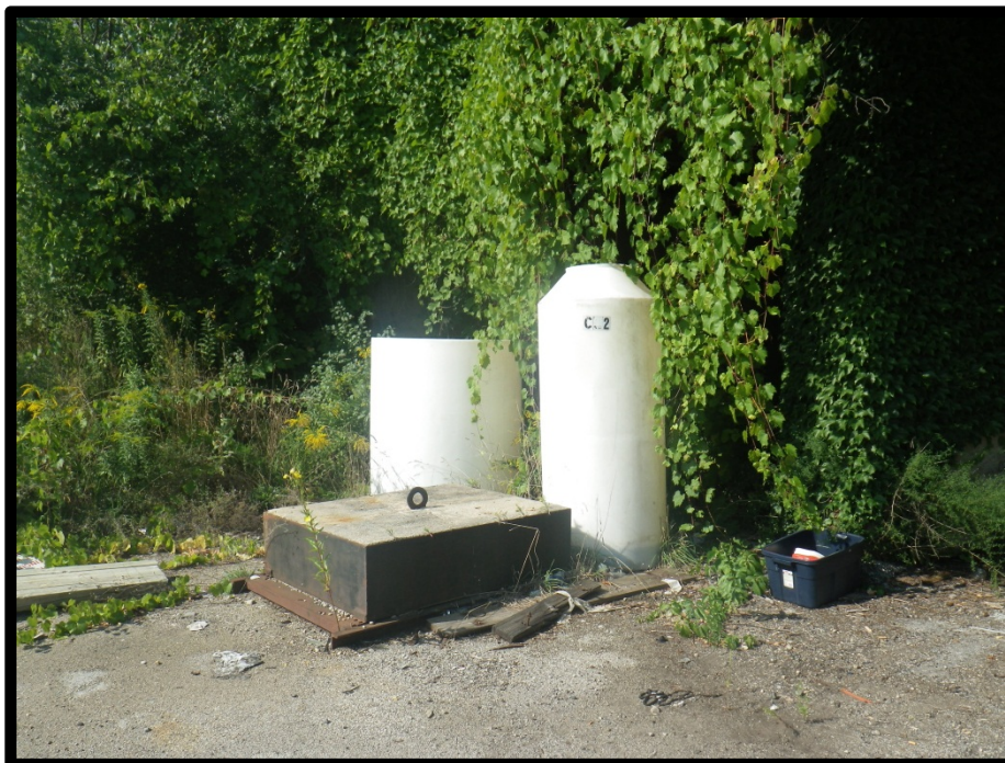
Empty ASTs located along the western side of the property.
