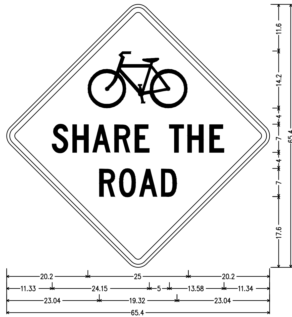
W21-6 MOD; 48.00" across sides 3.00" Radius, 1.25" Border, 0.75" Indent, Black on, Orange; Symbol RG025; "SHARE", C 2K; "THE", C 2K; "ROAD", C 2K;
