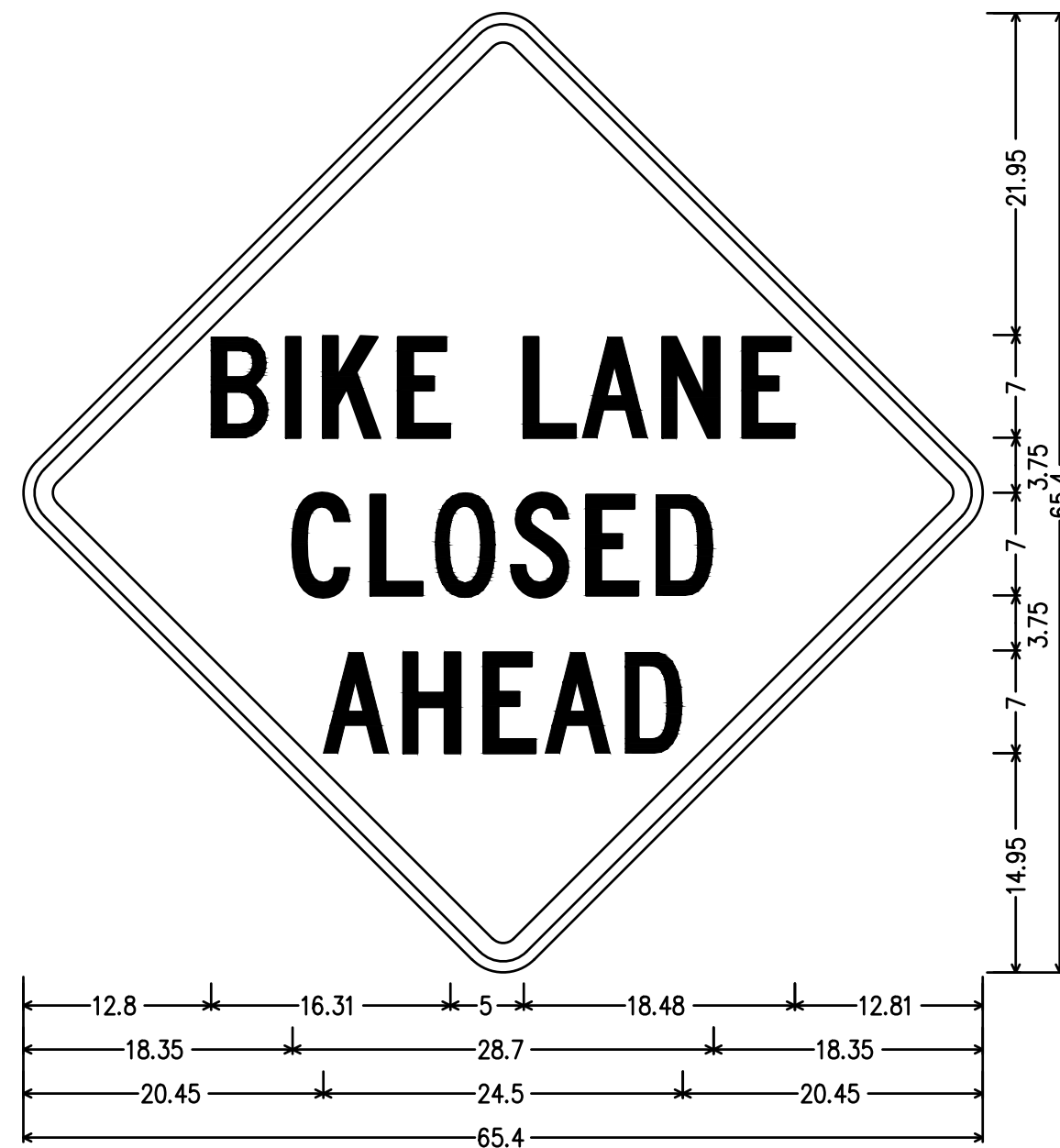
W20-5 MOD; 48.00" across sides 3.00" Radius, 1.25" Border, 0.75" Indent, Black on, Orange; "BIKE", C 2K; "LANE", C 2K; "CLOSED", C 2K; "AHEAD", C 2K;
