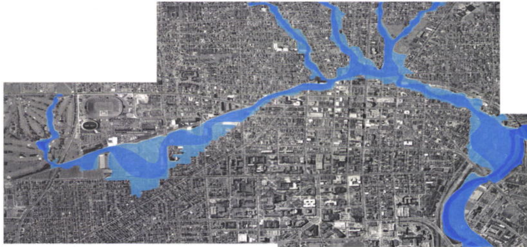
Figure 10: Allen Creek Floodway and Floodplain
