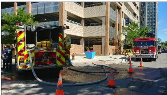
Engines are connected to a hydrant and then supply lines are hooked to the fire department connection to supply pressure for hose lines needed to extinguish vehicle fires.
