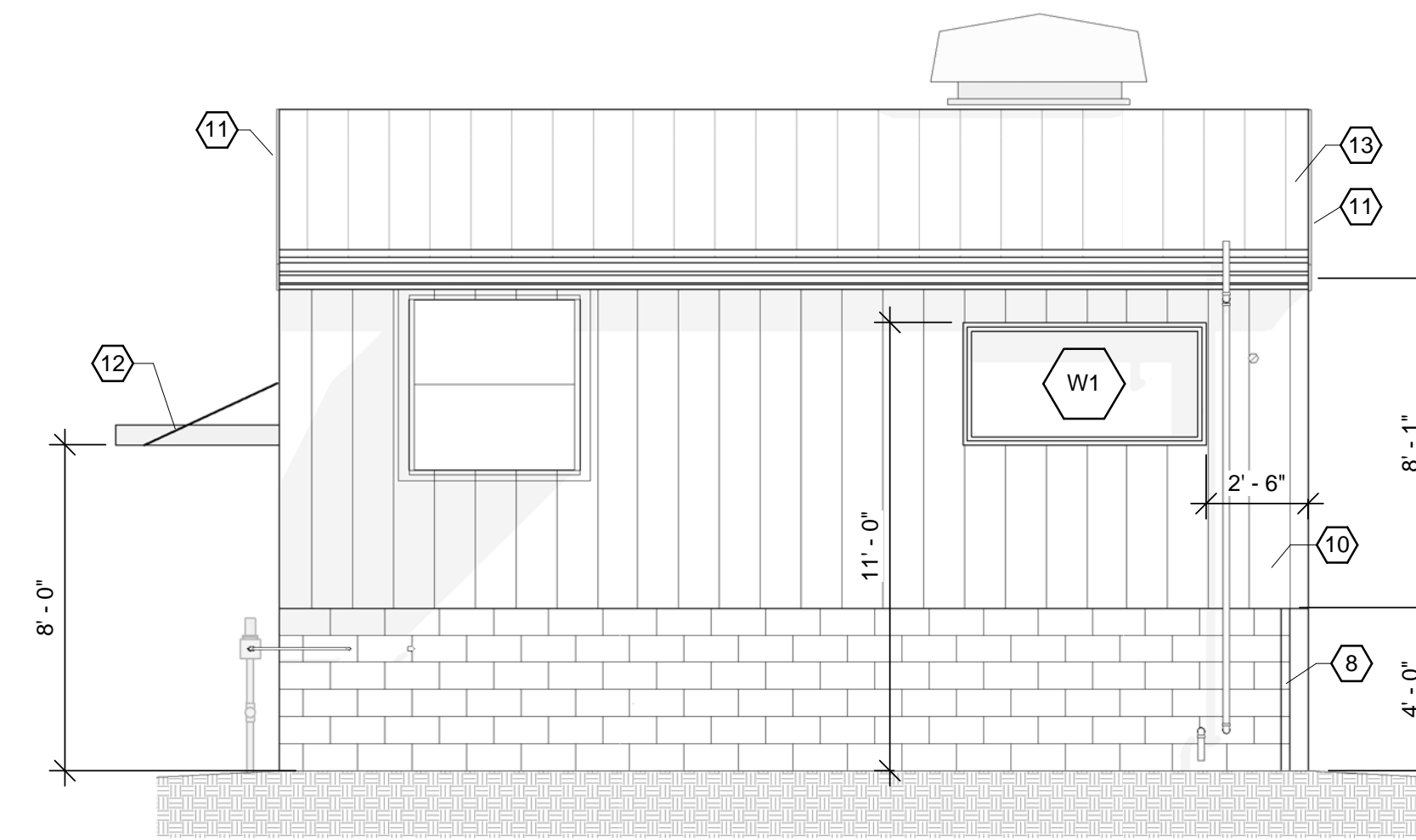
2 ELEVATION - WELL HOUSE 741 - EAST A-203 1/4" = 1'-0"
