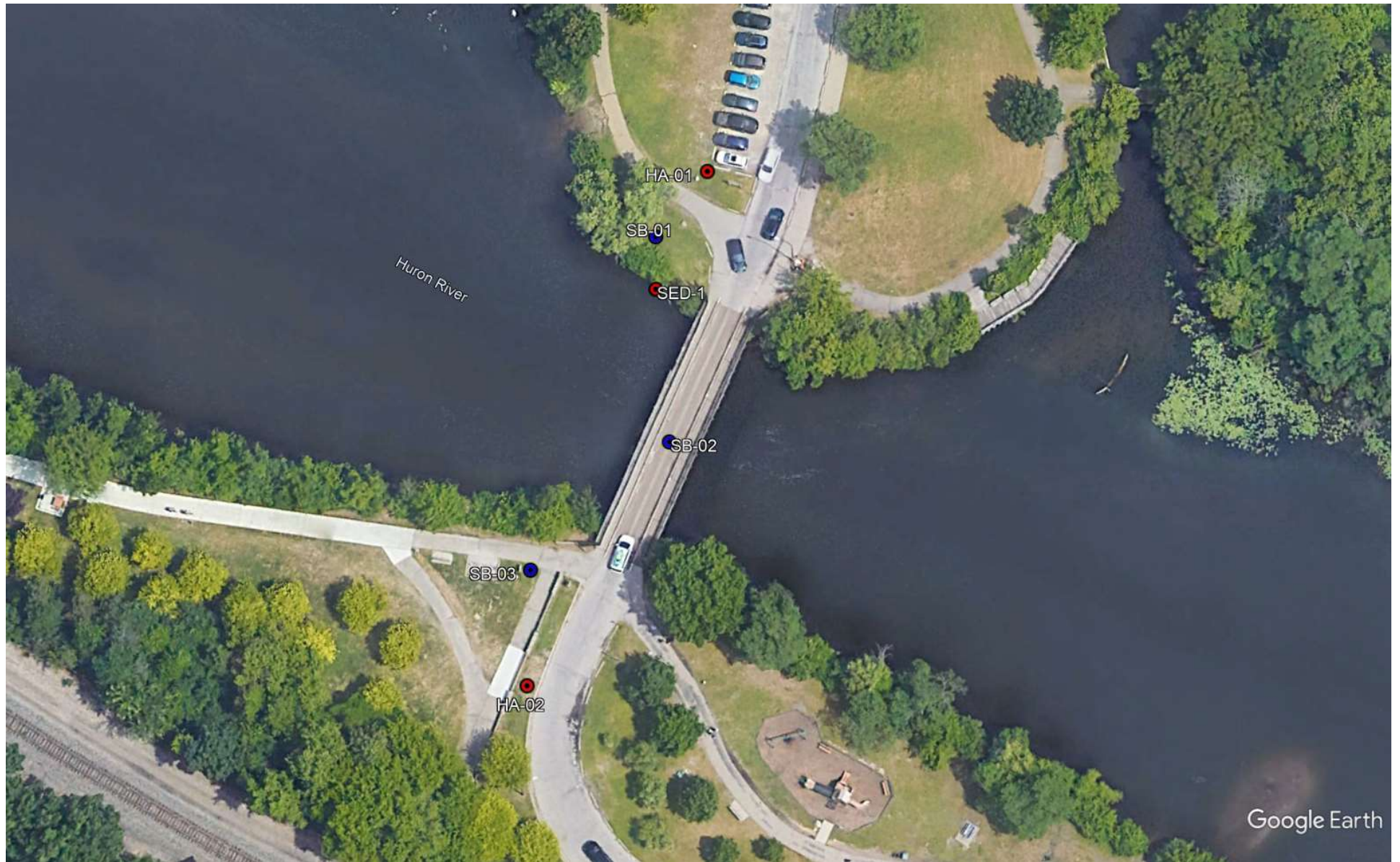
Figure 2: Soil Boring Location Map Gallup Park Bridge Replacement Ann Arbor, Michigan MSG Project Number: W2220001
