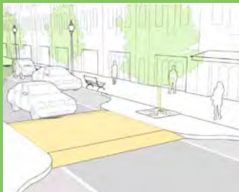
Figure 4-12. A rendering of a speed table, a design solution to increase safety where the trail crosses streets mid-block
