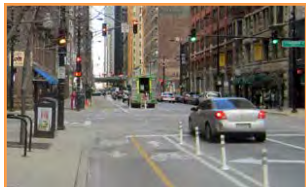
Figure 5-6. A dedicated bicycle stoplight gives cars a red arrow when bicyclists and pedestrians are crossing on the Dearborn Street cycle track in Chicago
