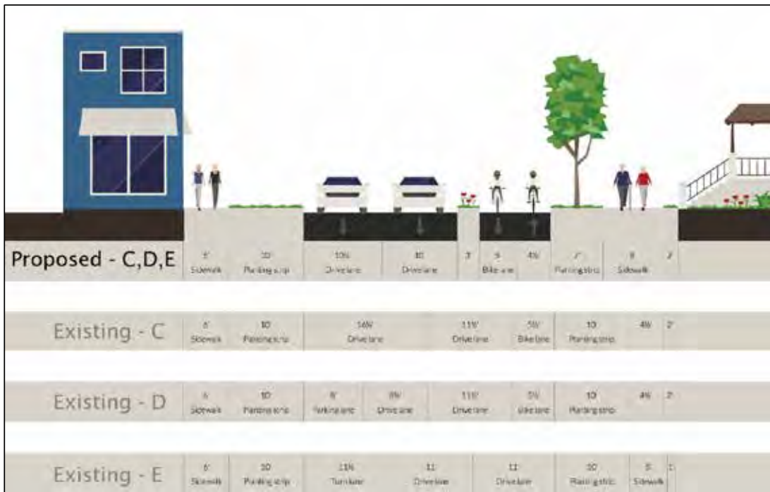
Figure 4: Cycle Track Sections C, D & E
