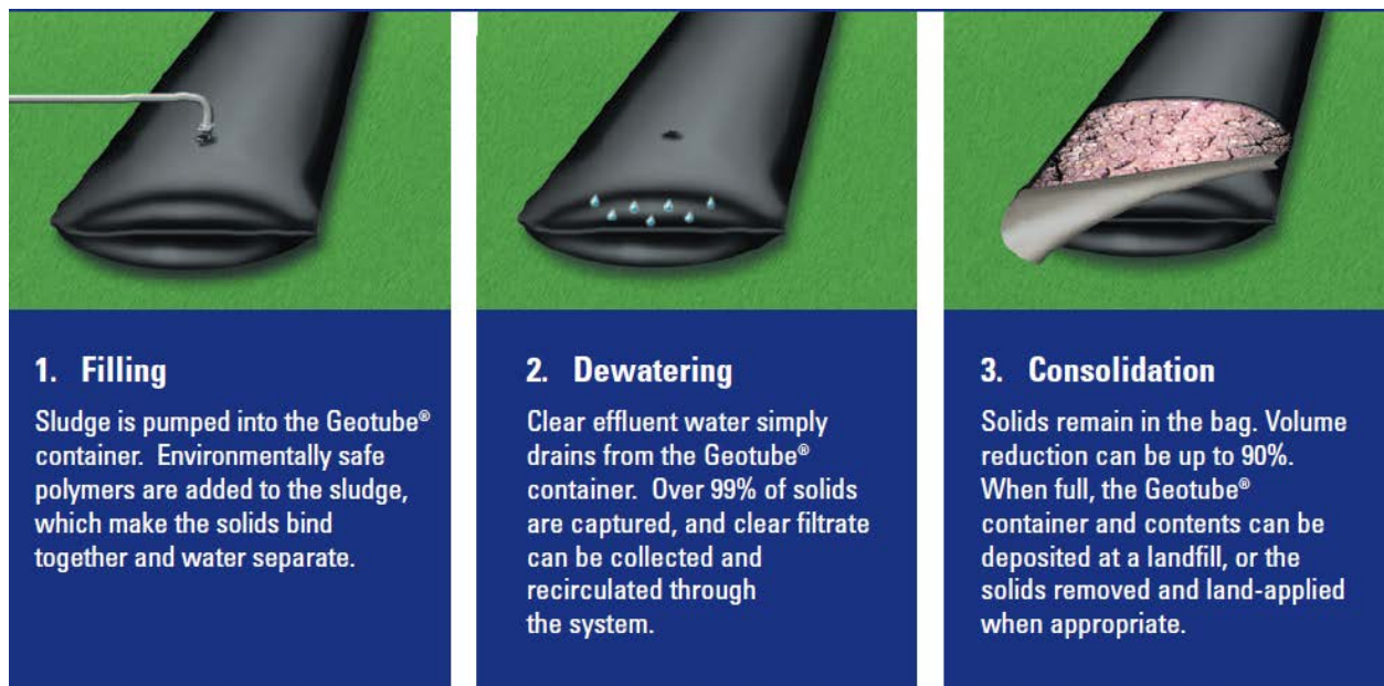
Figure TM4-14: TenCate Geotube Dewatering Technology
