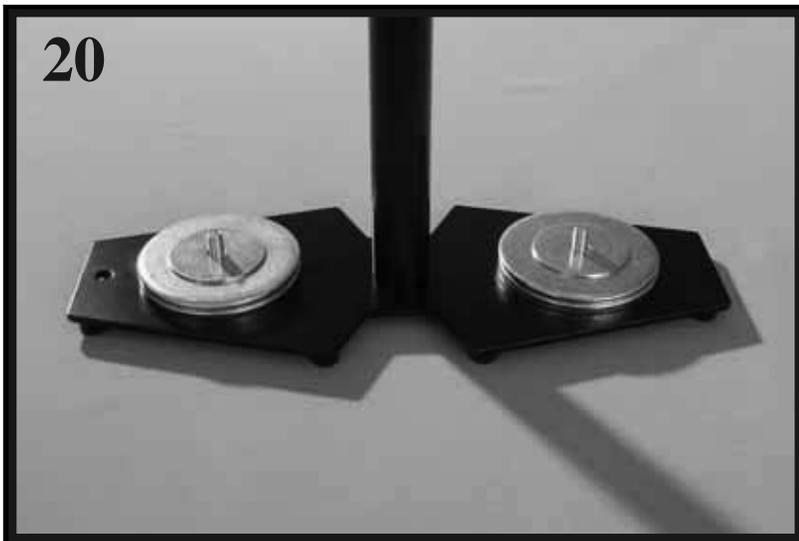
Place the two FENDER WASHERS over the COUNTER WEIGHT DISKS stacks as shown.
