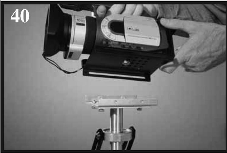
**NOTE:** Also, you could install a “Quick Release Plate” (not provided) between your Camera base and the HEAD PLATE at this time if you wish. We recommend the Bogen 3270, or 3273 “Quick Release Plates”. The Bogen 3273 is good for longer Cameras.
