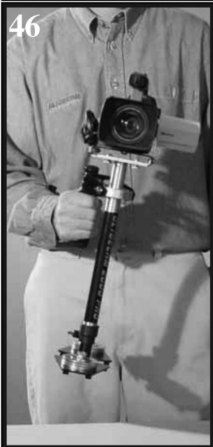
Also, another way of fine tuning the horizontal balance is to move the COUNTER WEIGHT DISKS back and forth, or side to side on the BASE PLATFORM. There are slots on the BASE PLATFORM to help with this task. Also, placing the WEIGHT DISKS away from the CENTER POST on the BASE PLATFORM will increase panning stability. Make sure to tighten the WEIGHTS down after you move them.
