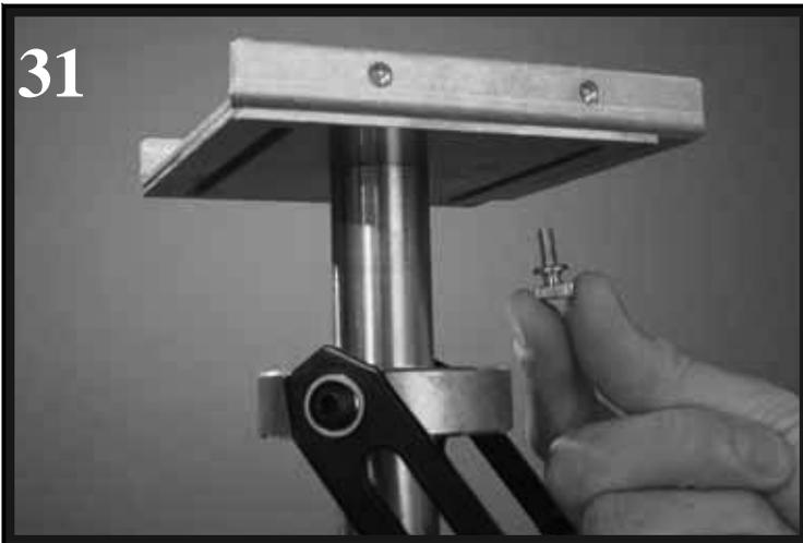
Insert the BRASS THUMB SCREWS through the slots in the BOTTOM PLATE and into the threaded inserts in the bottom of the MID PLATE.
