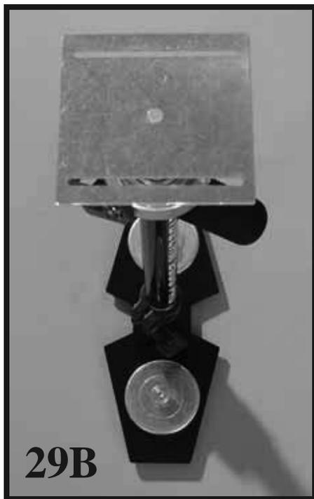
The **second** way to correctly align the parts (see Photo 29A) is to use a Phillips Screwdriver to loosen the “Screw” on the top part of the **TELESCOPING CLAMP** until you can rotate the parts so they are correctly aligned as in Photos 29B and 29C. Then simply retighten the “Screw”.
