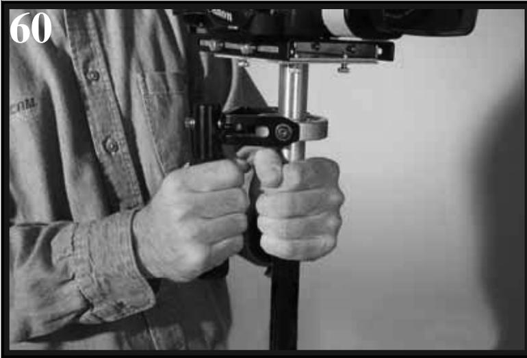
When shooting with the Glidecam 2000 Pro do not grab the **CENTRAL POST** as in Photo # 60, for this defeats the purpose and the isolation that the three axis gimbal provides. Instead handle your Glidecam 2000 Pro as shown in Photo # 51 and # 52.
