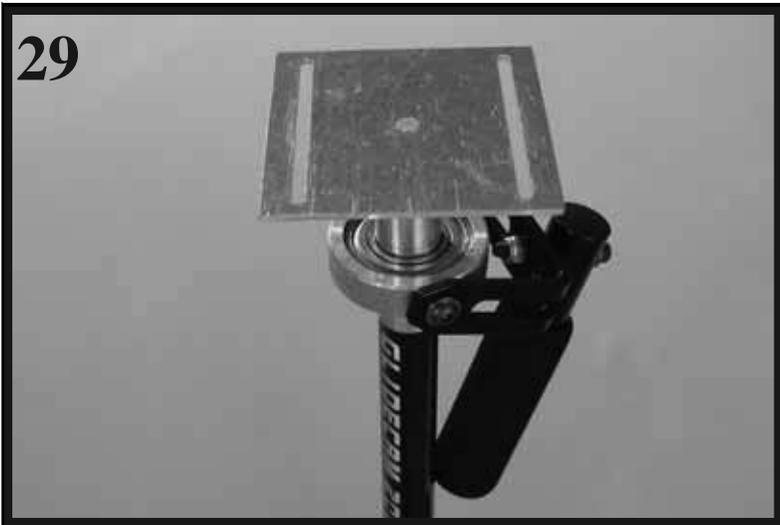
**Tighten** the **BOTTOM PLATE** to the top of **CENTRAL POST** to ensure a tight fit.
