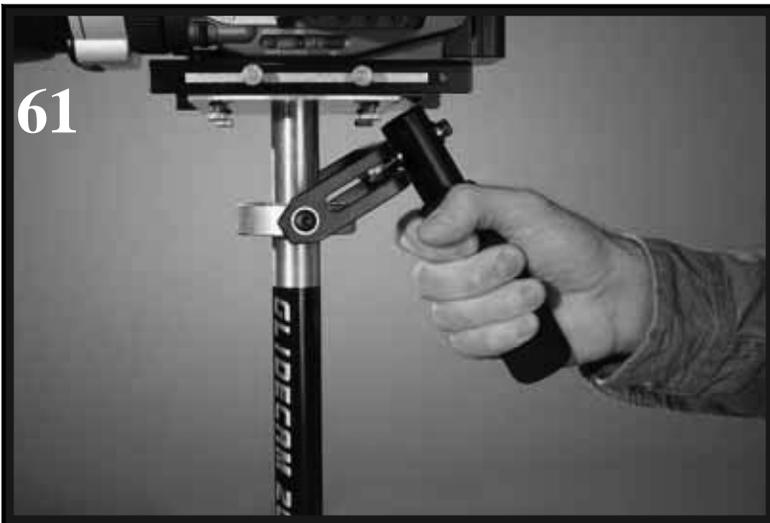
Do not allow the Handle of the Glidecam 2000 Pro to come in contact with the **BOTTOM PLATE** as in Photo # 61. If the Handle comes into contact with the **BOTTOM PLATE** it will limit your range of motion, and will result in “jerky”, and unpleasant footage. Instead position the Handle as shown in Photo # 50.
