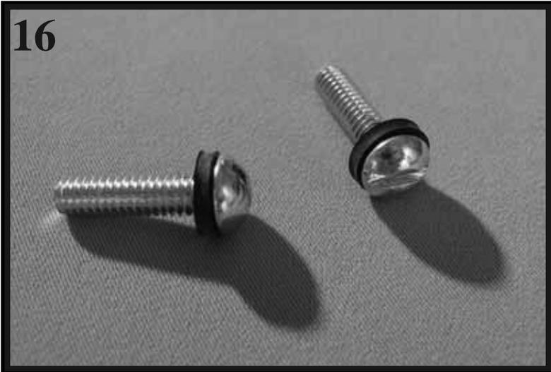
Now find a pair of bolts (example: 1/4" x 20 x 1") and attach RUBBER WASHERS as shown in the photo to the left.
