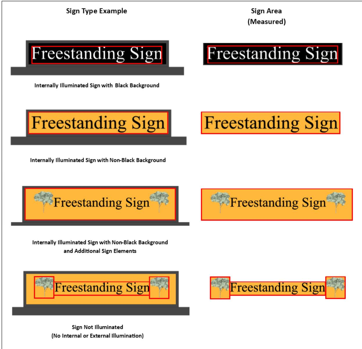
Figure 24-2: Calculating Sign Area of Wall Signs and Temporary Signs
