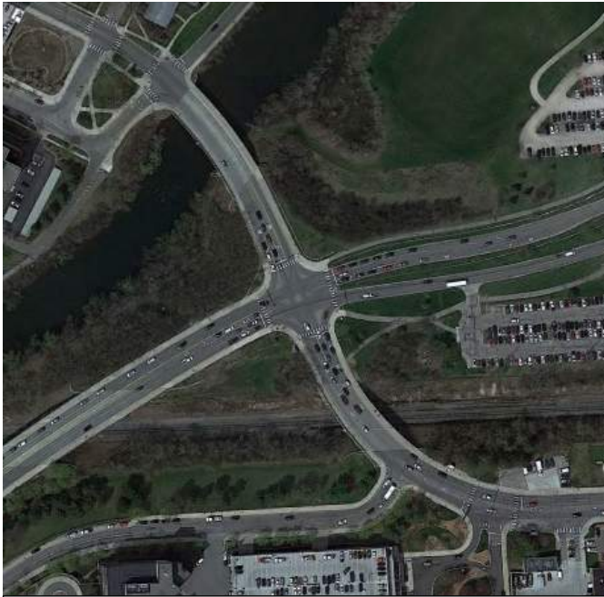
Figure 107: Fuller Rd at Maiden Ln/E Medical Ctr is highly congested with vehicles especially during the peak hours. Left turns from Maiden Lane onto Fuller Road cause backups during peaks.
