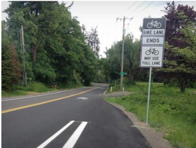
Figure 60: Add signs notifying cyclists and drivers to changes in bike infrastructure – Share the Road and Bike Lane Ends signs, where appropriate.
