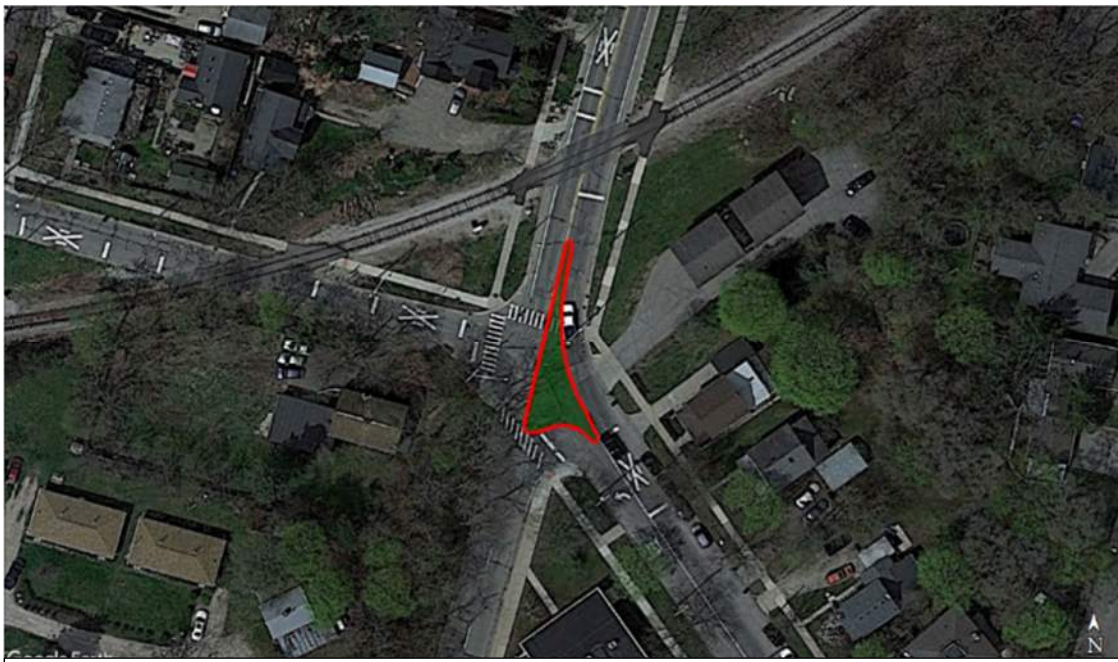
Figure 94: Mid-Term Option B – Add new island to intersection. Treatment would simplify the intersection by allowing only two movements from Moore Street and require Longshore to be right in/out only. Would remove traffic signals.
