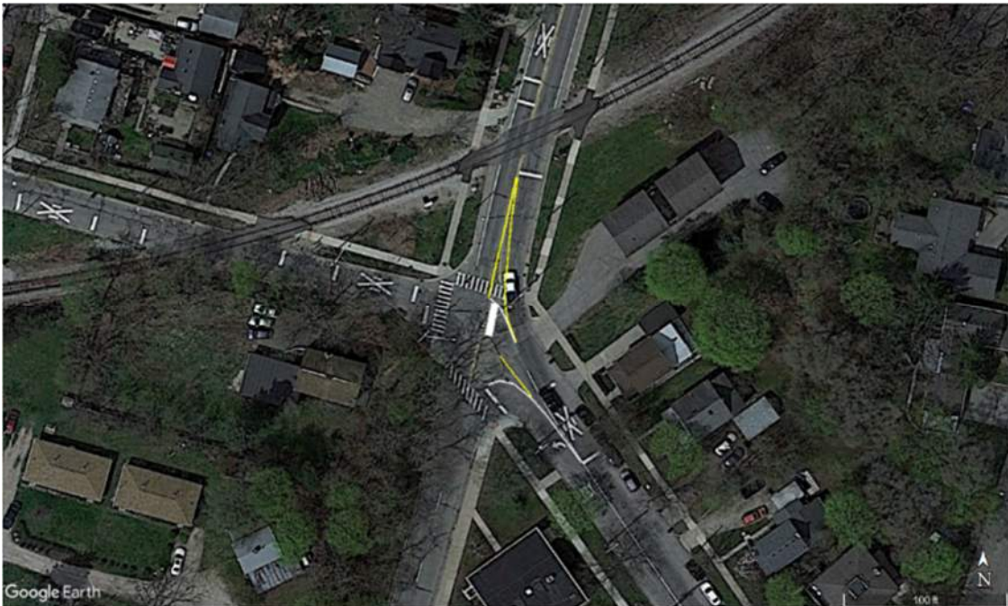
Figure 92: Short Term - Add pavement markings to better delineate vehicle paths through intersection. Maintain existing signals, but swap flashing yellow light for green arrow.
