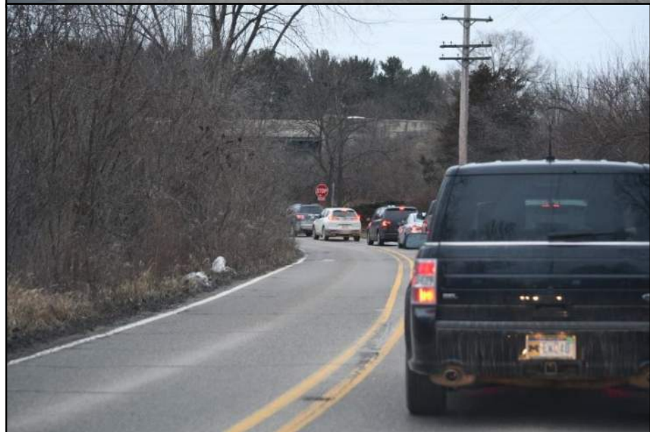
Figure 44: Queues on Barton Dr due to traffic seeking to enter EB M-14 generating backups down the ramp.
