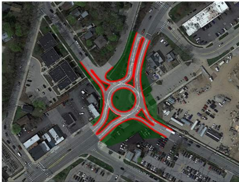
Figure 99: Convert intersection of Broadway St, Maiden Lane and Moore St to 2-lane roundabout. Moore St could change to 2-way traffic. Depicted is one with about 150' diameter.
