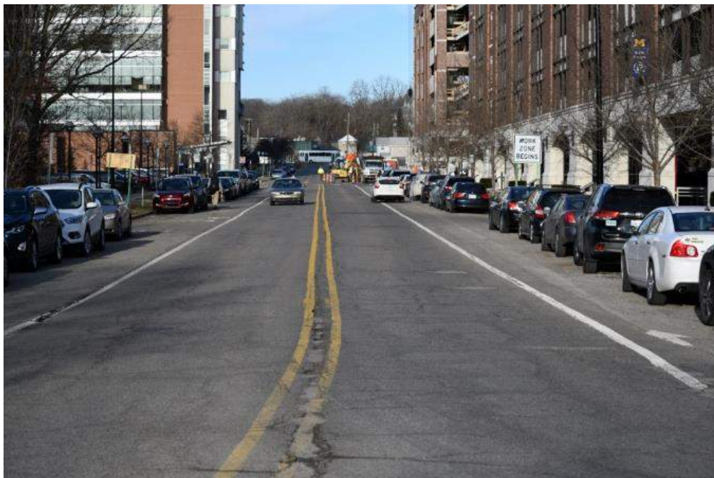
Figure 54: On-street bike lanes adjacent to parked vehicles should generally be wider (~6') to reduce likelihood of bicyclists running into opening car doors. Construction work zones must include warnings for cyclists that their exclusive lanes are blocked and there is a need to share the road. At least one instance of a car double-parked resulted in the bike lane being blocked.
