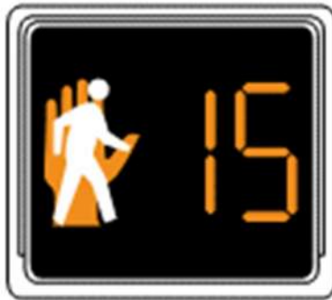
Figure 87: Accelerate the replacements of obsolete pedestrian signal heads. [Notes: MMUTCD Section 4E.07 – All pedestrian signal heads used at crosswalks where the pedestrian change interval is more than 7 seconds shall include a pedestrian change interval countdown display in order to inform pedestrians of the number of seconds remaining in the pedestrian change interval. There was an August 2015 compliance date for the replacement of all pedestrian signal heads at such locations to incorporate the countdown feature. This may imperil agencies receiving Act 51 funding.]
