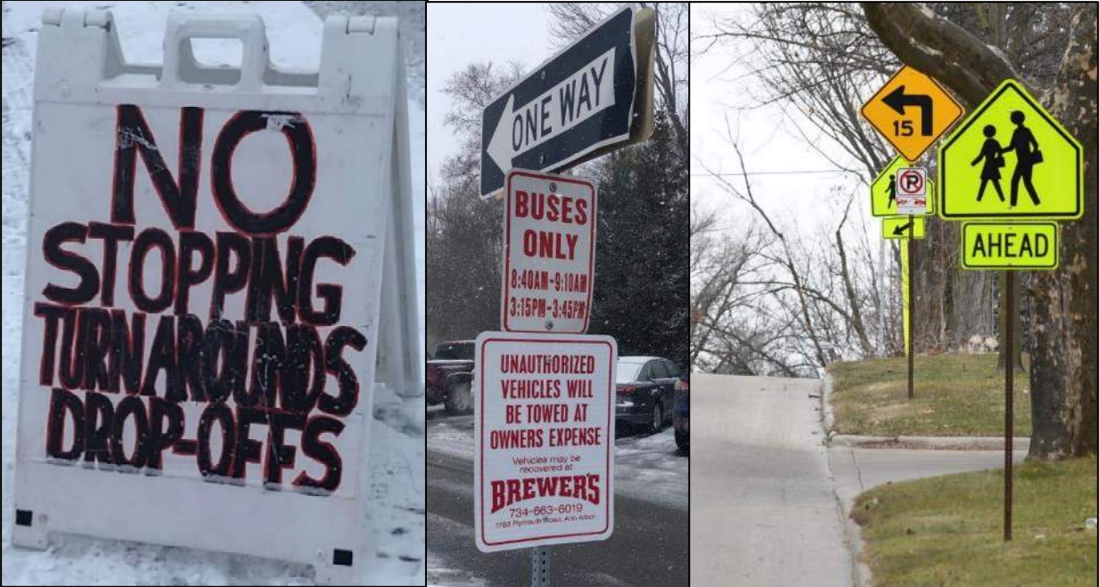
Figure 116: Signing practices around the school are confusing and not to roadway standards. Some signs are handmade, others are typical standard street signs but poorly located, and others are related to towing practices.
