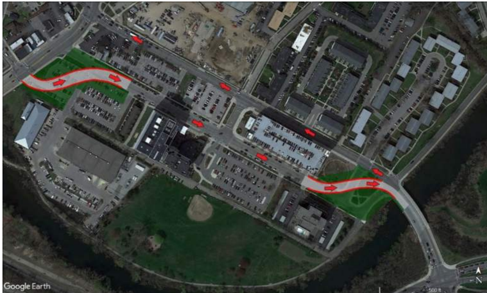
Figure 100: Convert Maiden Ln and Wall St to one-way pair. Option A: Shift western portion of Wall St to align with Swift St at signalized intersection and eastern portion to join Maiden Ln prior to Huron River bridge. One-way pair has less conflict than two-way operations. Reduces operational stresses at Broadway Street/Moore Street/Maiden Lane intersection. Driving lanes, bike lanes, and Wall Street parking lane would all fit into the cross section for both streets.
