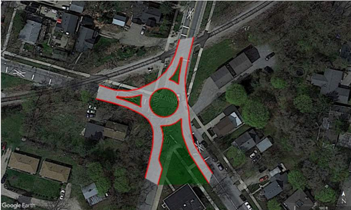
Figure 95: Long Term – Reconfigure intersection as one-lane roundabout. Maintains access for all existing movements. Would eliminate all signals. Depicted is one with about 90' diameter.
