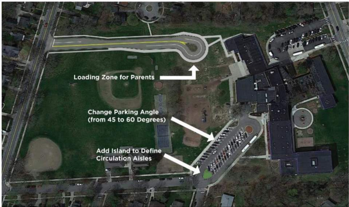
Figure 118: On-Site Changes – Build a new driveway off Pontiac Trail to function as a loading zone for parents to easily and safely drop off students at the school. In the parking lot on the west side of the school building, accessible via Taylor Street, the parking spaces could be changed from 45 degrees to 60 degrees to allow room for more spaces. Build an island at the end of this parking lot to better define the circulation aisles and the intersection of Taylor St, Peach St and the school drive.
