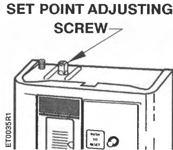
Figure 4. Set Point Adjustment Screw.
